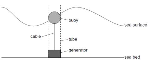
The motion of the buoy can be assumed to be simple harmonic.
